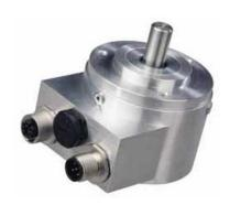
These "Outdoor encoder" is suitable for harsh industrial environments. The heavy-duty option for the CANopen encoder provides a wide temperature range, protection elements against perspiration water inside the encoder and a heavy-duty housing. Uppermost attention was laid on a high EMI protection. Micro style connectors for power supply and bus-in / bus-out
